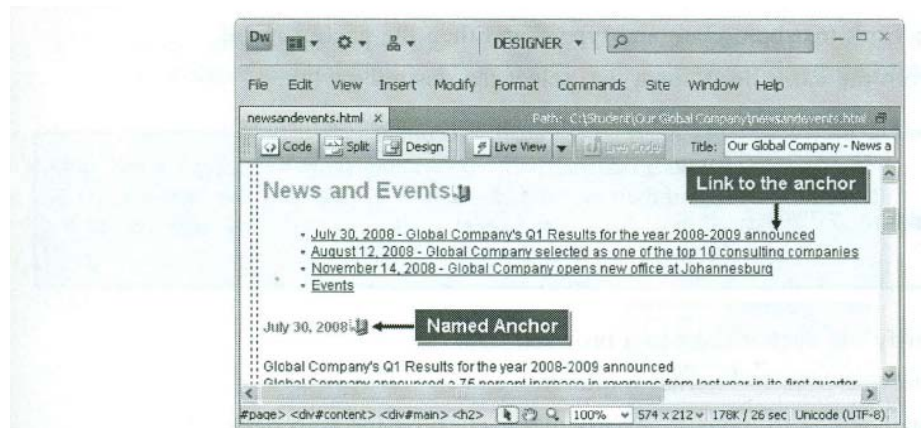
Figure 5-1: A web page displaying an anchor and a link to the anchor.
